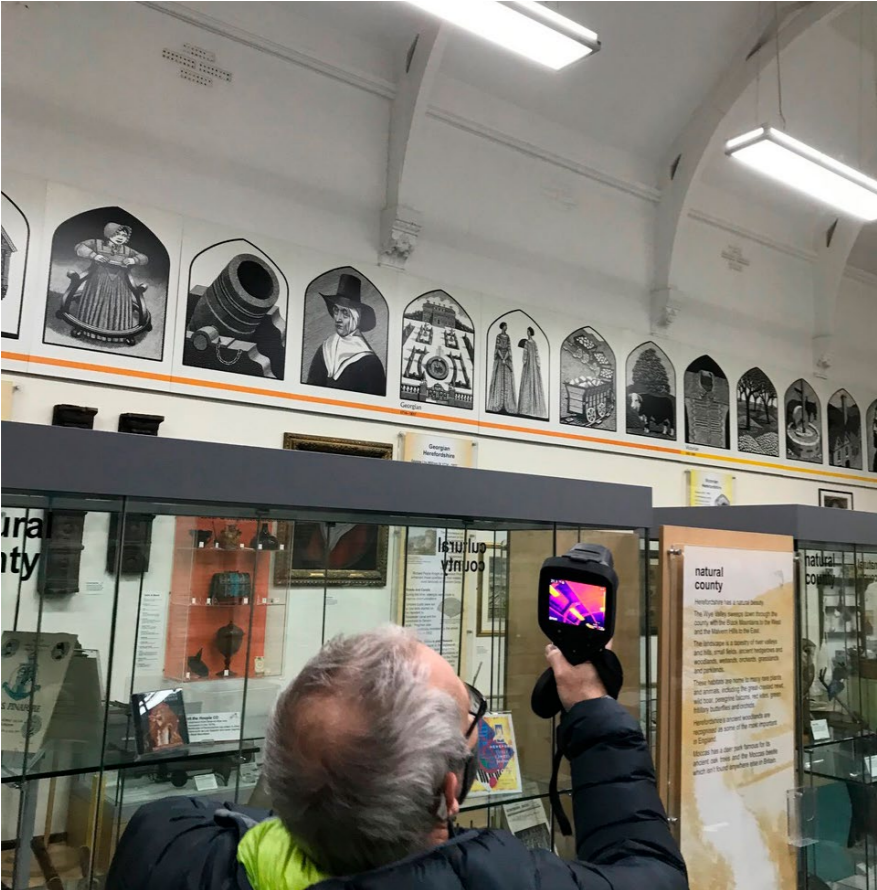
Fig. 91 / Forensic Investigation / Thermography camera highlights original roof lights in Museum space. Source: Architype, 2021.
